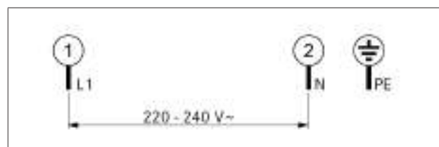
Fig. 4.86 1-phase connection diagram
